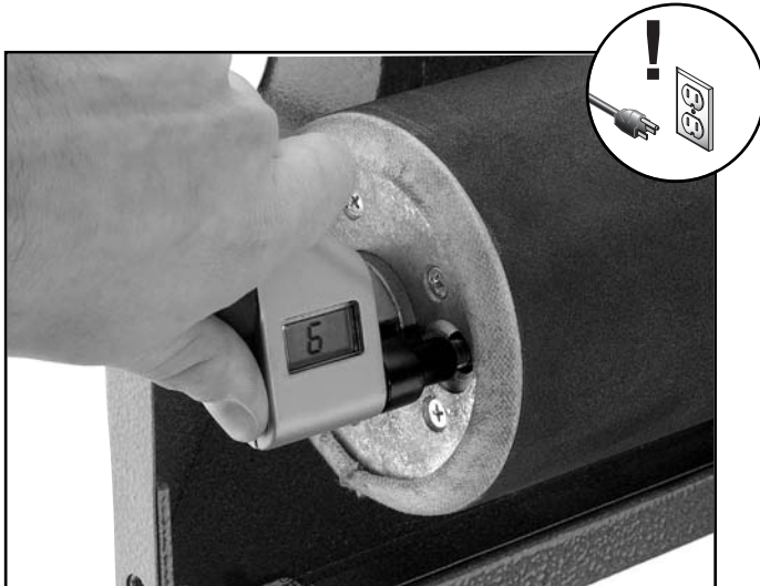
Figure 20. Checking air pressure.
